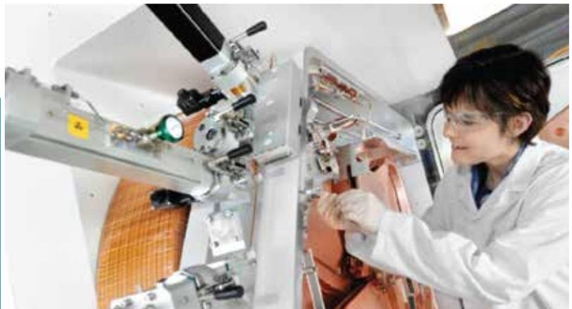
*On-site maintenance of a cyclotron by a technician*
